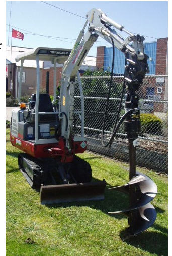
Takeuchi 1.6 tonne Excavator with the Posthole attachment.
