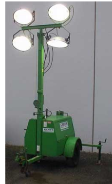
Diesel Lighting Tower
