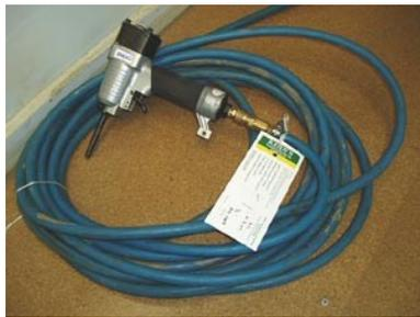
**Basso Nail Puncher make light work of the hard job of punching nails down.**
