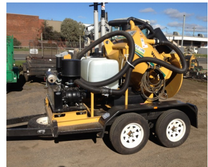
Vermeer Vacuum Excavator
